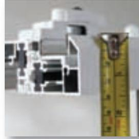
The slimmest of meeting rails preferred by customers and local planners is just 36mm. Clever profile design and bonded glass to the sash gives incredible strength. More glass area, less frame and is close to the original wooden box sash window look, allowing better thermal performance. Within the meeting rail is a radical box and 'T' design, which resists deflection or bow.
