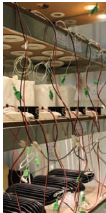
Quality LED products on test for 6,000 hours at an ambient temperature of 25°C
