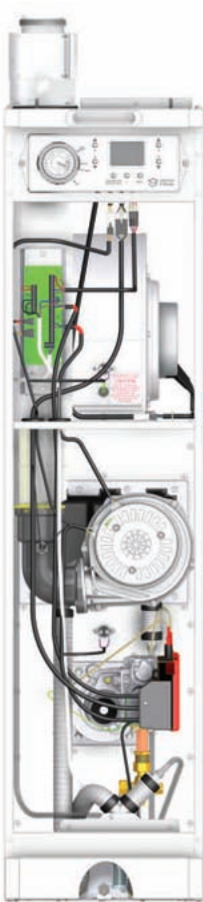
Internal view diagram of condensing air heater, a highly efficient condensing gas fired downflow forced convection air heater
