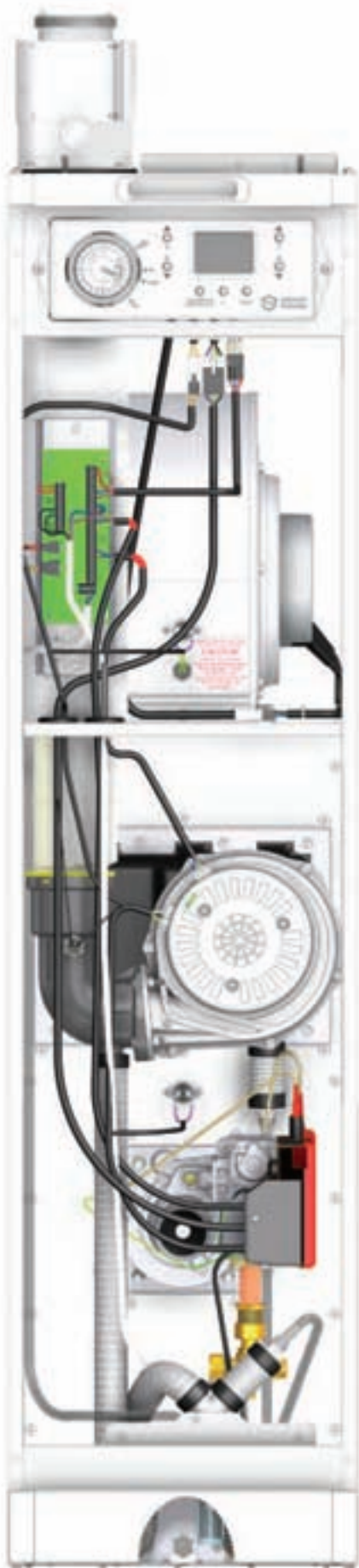
Internal view diagram of condensing air heater; a highly efficient condensing gas fired downflow forced convection air heater
