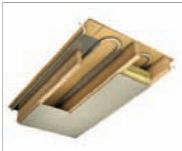
Cross section schematic drawing of a specialist metal heat diffuser plate system, which is ideal for use in suspended timber floors. The plates can be fitted from above on top of joists where the existing floor is being lifted or between the joists from below if ceilings are being replaced
