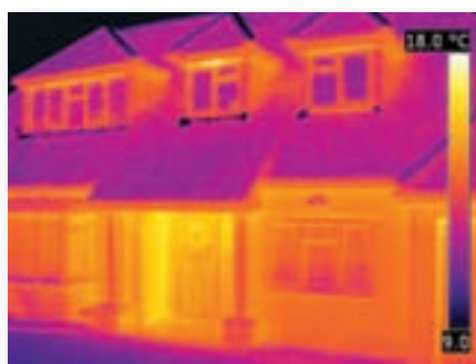
THERMAL IMAGERY SHOTS TAKEN IN CONJUNCTION WITH AN AIRTIGHTNESS TEST SHOW THE EFFECTIVENESS OF MEASURES TAKEN
