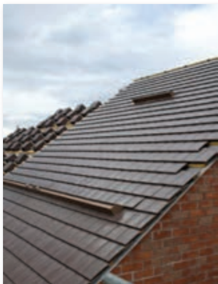
THIS RAINWATER HARVESTING SYSTEM USES RAINWATER COLLECTORS PLACED ACROSS THE WIDTH OF THE ROOF AND INTEGRATED WITH THE TILES. EACH COLLECTOR FEATURES A SELF-CLEANING FILTER THAT FILTERS THE RAINWATER BEFORE IT IS DIRECTED TO THE STORAGE TANK IN THE LOFT SPACE
