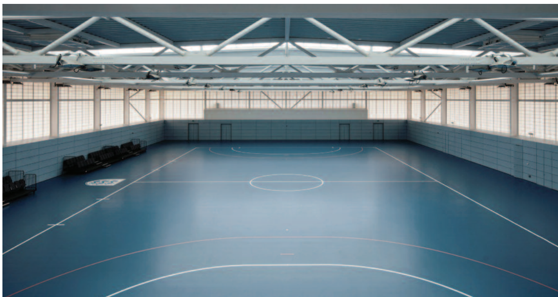
Pictured: Used in FA's St George's Park football centre, by RedBox Design, Kalwall with integral aerogel, has an insulation U value of up to 0.28W/m 2 K making it almost as effective as a solid wall
