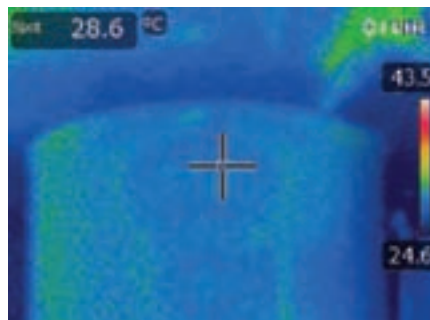
Thermal image of cylinder with side mounted hot water outlet
