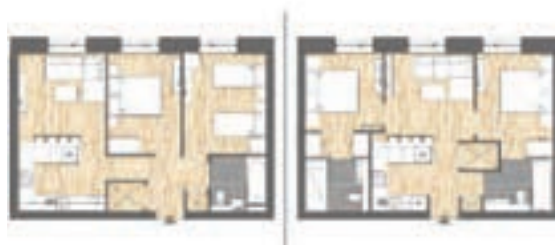
Layout comparison of typical for sale unit (left) and typical build to rent unit (right) © Geraghty Taylor Architects
