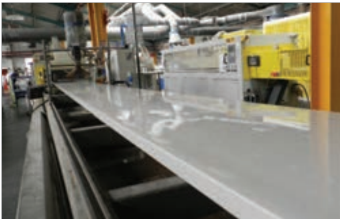
Production of cellular PVC fascia boards
