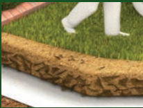
TRACKTURF Reinforcement Reinforced grass surface using rootzone & plastic elements.
