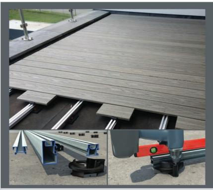
Designed for use on flat roofs and balconies for the installation of decking and porcelain tiles. The beams are available in three sizes to accommodate different threshold restrictions and span requirements. Fasteners are available to secure the decking or porcelain paving to the aluminium
