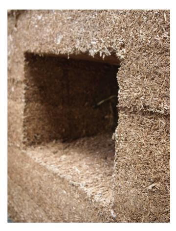
An opening in the thermal layer of the new CobBauge material All Images © University of Plymouth
