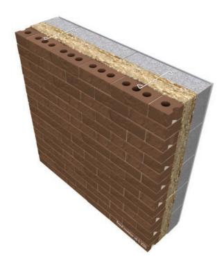
Beyond the thermal, fire and acoustic performance considerations, providing ease of correct installation should be top of mind. For example, during installation, mineral wool insulation products adapt to imperfections in the substrate
