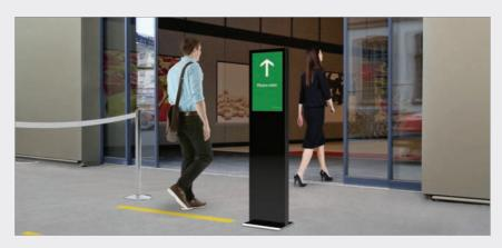
environment for everyone." In addition to closing the doors when the maximum number of people entering an area has been reached, TORMAX count+go issues a clear acoustic signal to alert pedestrians to wait. As soon a person exits the building, bringing the number back down, the door returns to the open operating mode.
