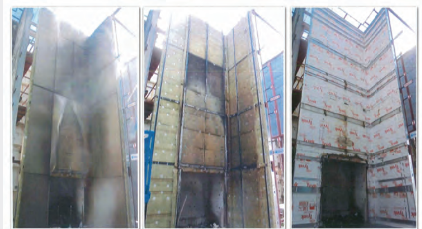
Anodised Aluminium Sheet - tested to BS 8414
