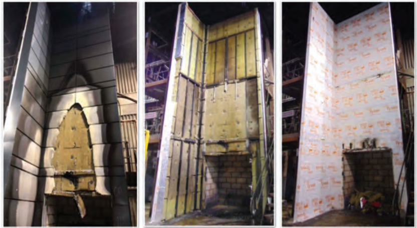
PPC Aluminium Sheet - tested to BS 8414
