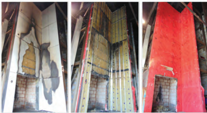
Pre-Coat Aluminium Sheet - tested to BS 8414
