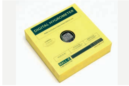
A calibrated hygrometer – for measuring subfloor relative humidity
